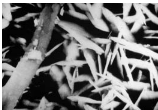
Figure 4. Gypsum crust formation.
