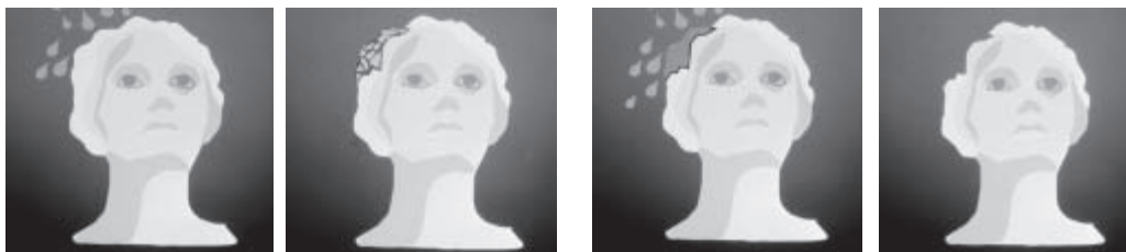
Figure 2. Deterioration of limestone caused by wet deposition of sulfur dioxide.
